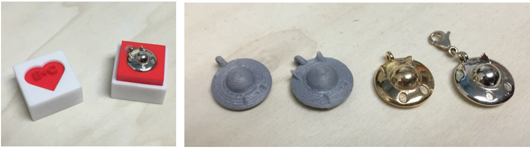
Figure 4. Calvin and Hobbes charm designed and prototyped in Jumbo's Maker Studio. (Left) 14k white gold charm in nylon case, both printed at shapeways.com. (Right) From right to left: PLA and ABS prototype printed at Jumbo's Maker Studio, brass and white gold versions printed at shapeways.com
