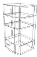
This differentiated design improves the refrigerators energy use impact (as measured by  $\rm CO_2$ ) by 22.6%. This design allows for reduced lifetime costs because it allows for portions of the refrigerator to be kept at higher temperatures based on recommended food storage guidelines, thus requiring less energy to operate. It also allows the user to turn off sections completely when not in use, saving even more energy.
